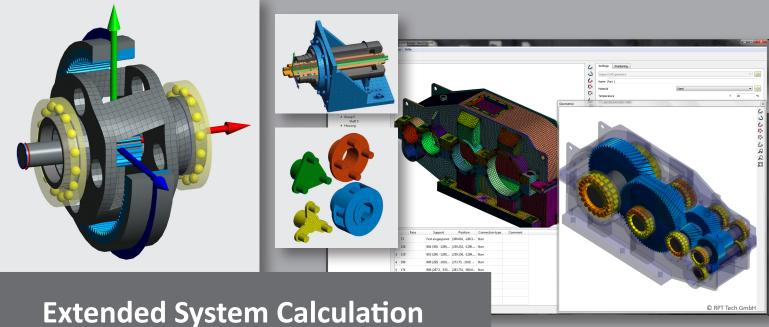
*SystemManager* software allows for a fast and easy design of complete systems of machine elements. The individual system elements are directly linked to the eAssistant/TBK calculation modules. Listed below is an overview of some of the major new features in version 04/2017:
